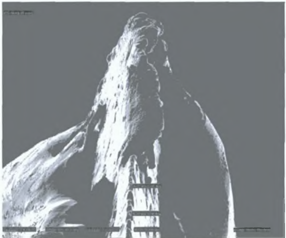
Figure 2.2 Scalpel blade edge, field of view 20\mu\text{m} , annotated radii 0.21 - 0.31\mu\text{m} , source MDW Technologies ( http://www.mdwtech.com/imaging/images.html )
