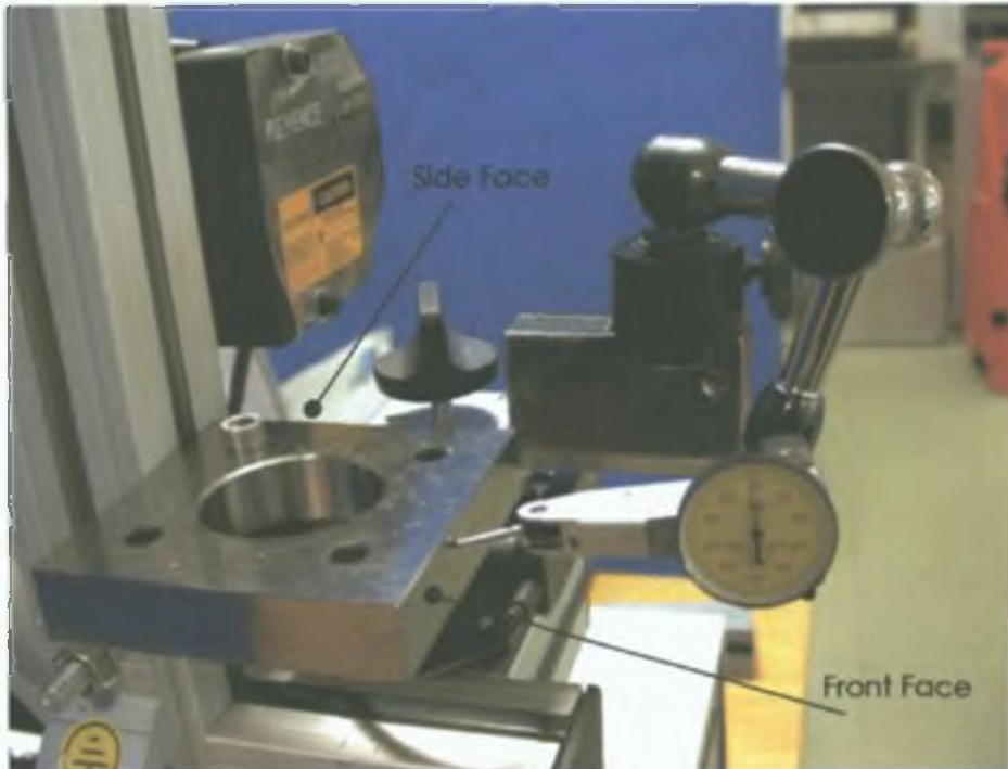
Figure 4.20 Aligning the slides using dial gauge
