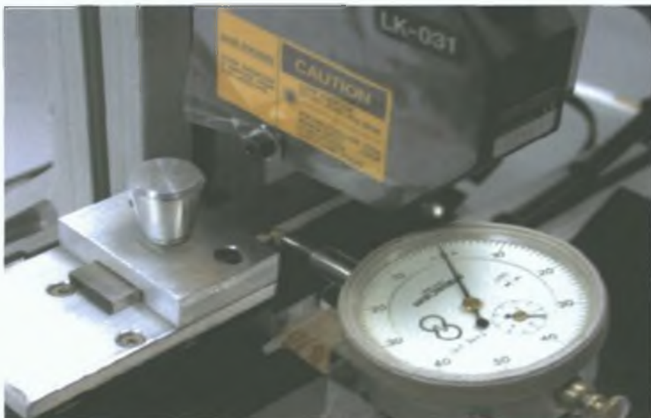
Figure 4.21 Aligning the clamp unit using dial gauge
