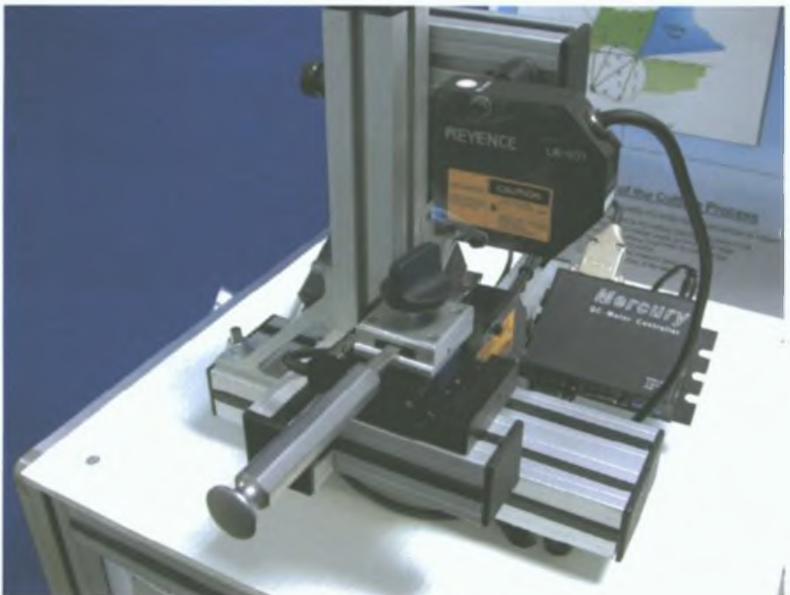
Figure 5.19 12mm osteotome set up for scanning
