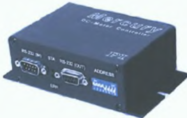
Figure 4.22 Mercury II C-862 single-axis DC-motor controller
