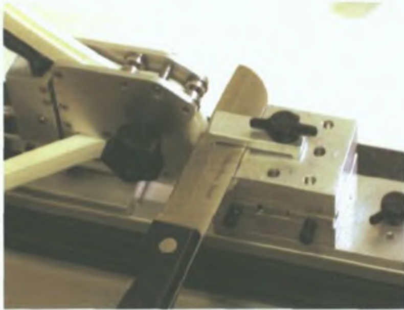
Figure 3.5 CATRA sharpness tester, force based test.
