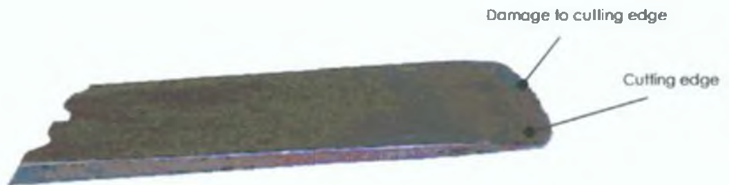
Figure 1.7 Osteotome removed from service, showing signs of chipping of the blade tip, this particular osteotome should not have been used, hence the requirement for procedures for the inspection and maintenance of surgical cutting equipment
