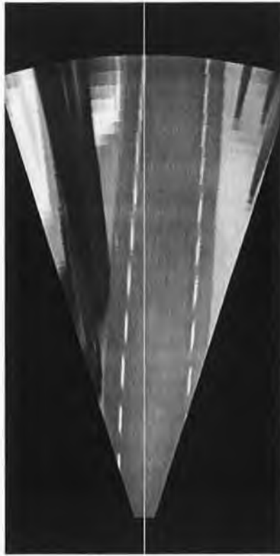
Figure 26. Corrected image after Inverse Perspective Algorithm has been applied
