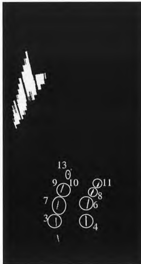
Figure 49. All the detected Left and Right markers in image of roadway halfway through S-bend.
