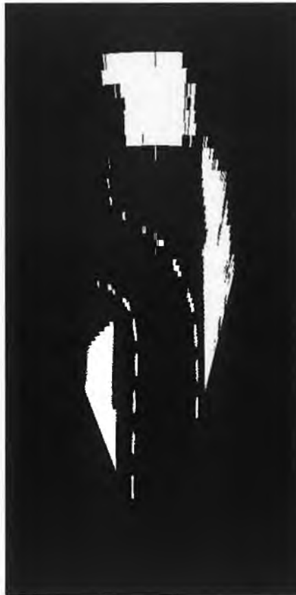
Figure 47. Roadway with S-bend ahead, after Threshold Operation.
