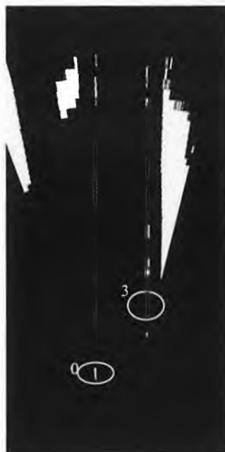
Figure 44. Finding the first lane markers on left and right sides of the lane.
