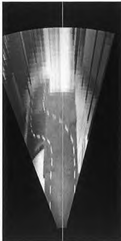
Figure 36. S-bend section of roadway after Inverse Perspective Algorithm applied.
