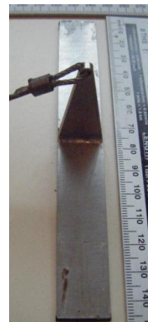
Figure 3-28 Plate Anchor e/B = 2 (Photo)
