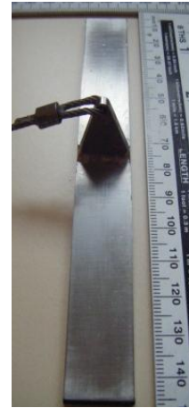
Figure 3-24 Plate Anchor e/B = 1 (Photo)
