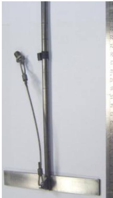
Figure 3-33 Mandrel used to Install the Plate Anchor
