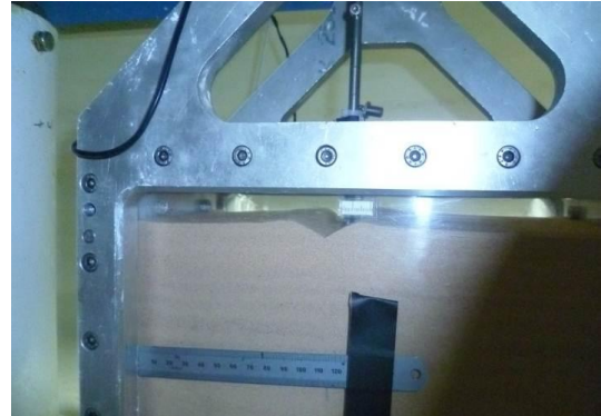
Figure 5. Anchor installation at 1 g showing disturbance of the sample surface
