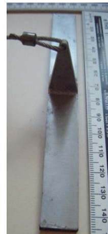
Figure 3-26 Plate Anchor e/B = 1.5 (Photo)
