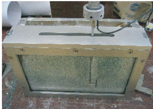
Figure 2-3 Testing Chamber with Installed Anchor (after O'Loughlin et al. 2006)
