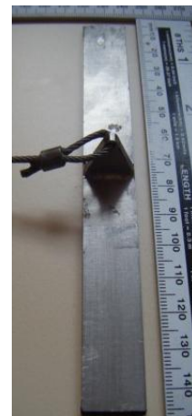
Figure 3-22 Plate Anchor e/B = 0.75 (Photo)
