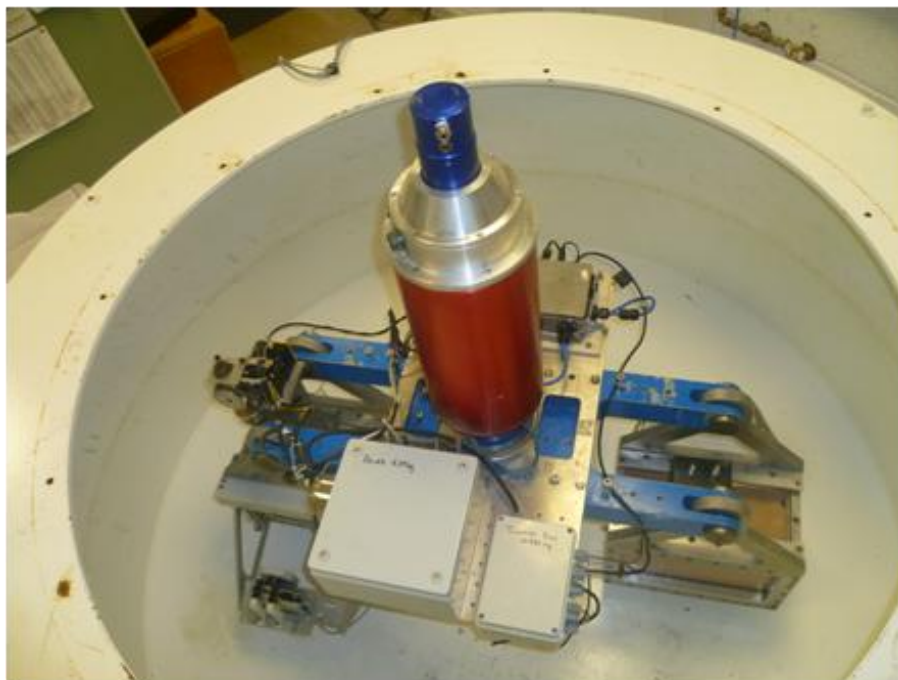
Figure 3-2 Internal View of Centrifuge in Beam Mode – Loading
