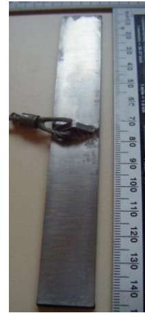
Figure 3-18 Plate Anchor e/B = 0.25 (Photo)
