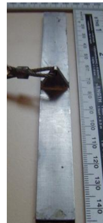
Figure 3-20 Plate Anchor e/B = 0.5 (Photo)
