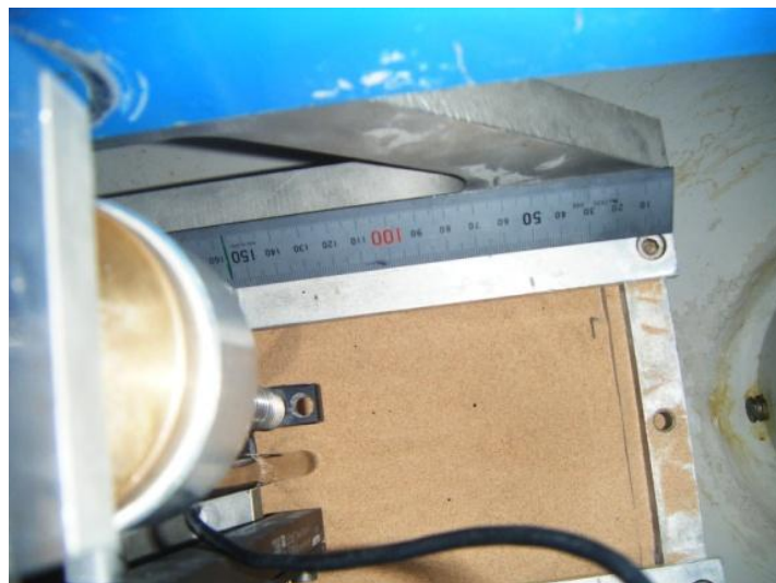
Figure 3-31 Installation of Cone Penetrometer (a) Side view of cone penetrometer (b) Side view of CPT setup (c) Plan view positioning actuator
