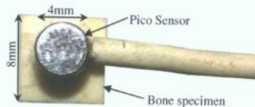
Figure 3.8: AE sensor placed on the bone specimen
