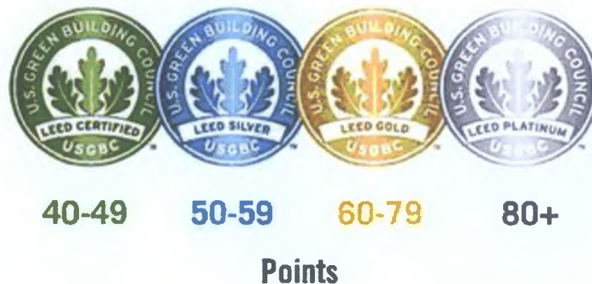
Figure 4: Four Certification Levels (source: LEED (2009) Four Certification Levels, Core Concepts and Strategies ).
