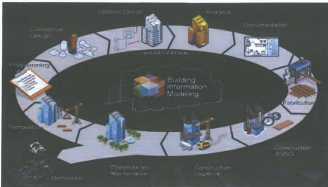
Figure 2: The Daily Life of Building Information Modelling, Phases of a BIM project Lifecycle (Dispenza, 2010)
