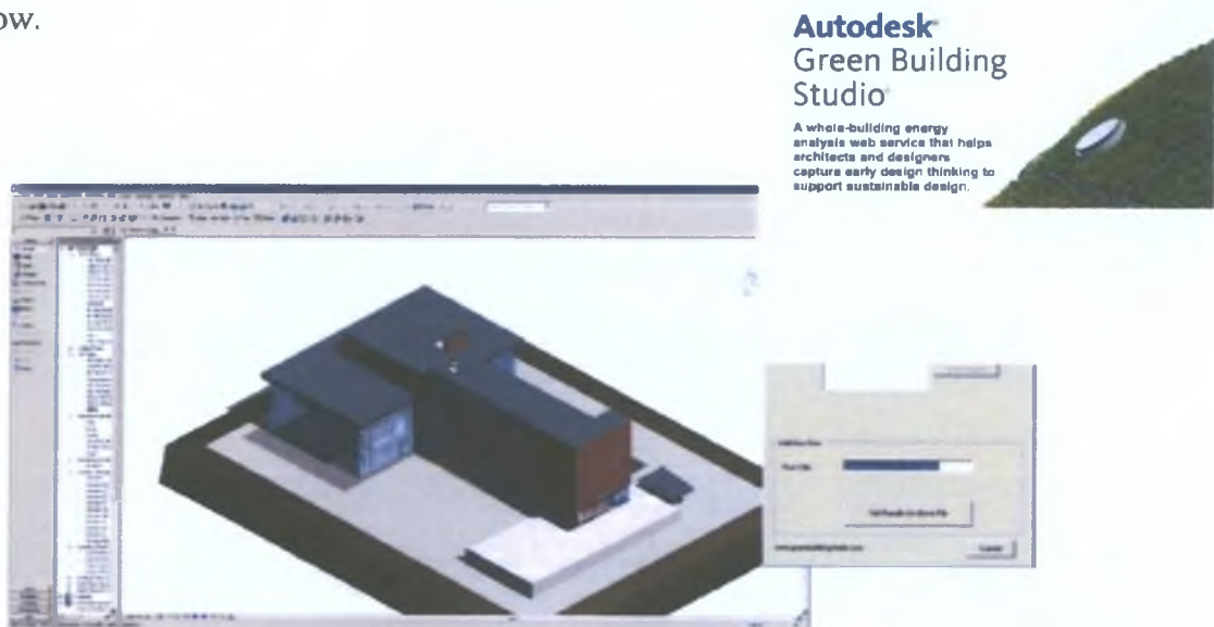
Figure 8: The link between the Revit platform and the Autodesk Green Building Studio web-based service is facilitated through a plug-in that enables registered users to access the service directly from their Autodesk Revit Architecture design environment.
