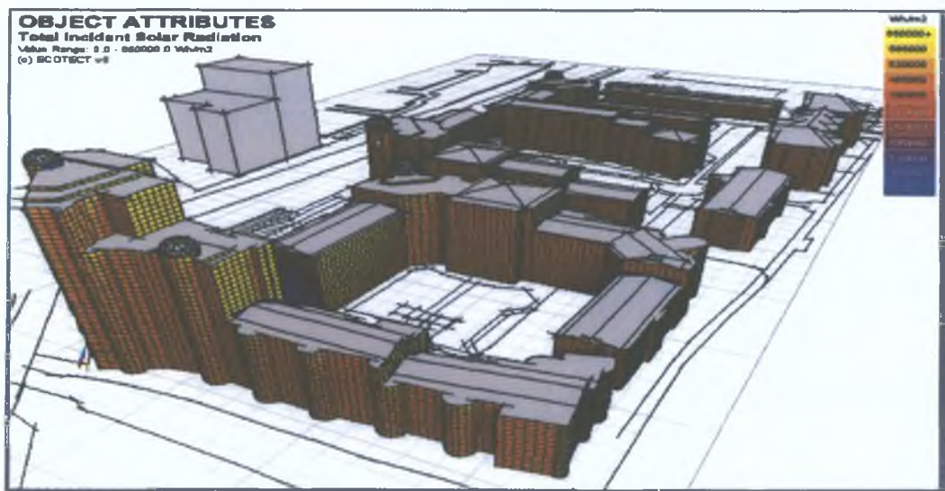
Figure 15: Using Autodesk Ecotect Analysis, architects can see the results of their analysis displayed in the context of a building model, such as the surface-mapped results of this solar radiation analysis .
