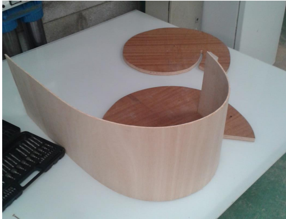
Figure A.1: Securing the flexible plywood to the template as per Step 5.
