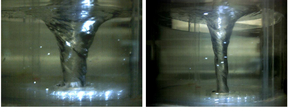
Figure 5.16: Particle images using the PSV method for (a) h/d = 2 and (b) h/d = 3.5 in model #4.0d1.5d and #5.0d2.0d respectively. Figure 5.17(b) shows the particle streaks when aligned with the x_0 - z_0 plane as discussed in section 5.7.2.
