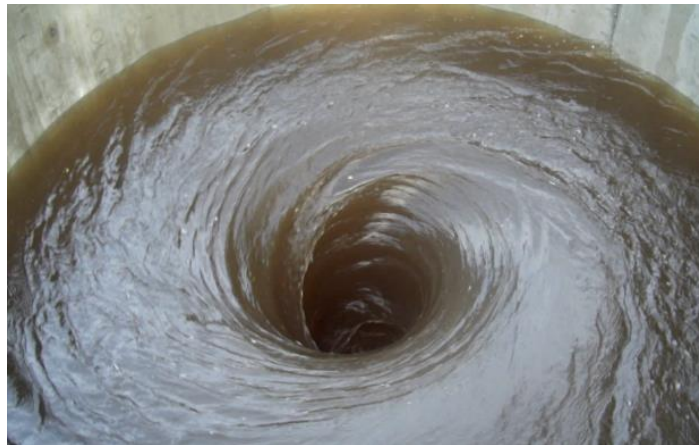
Figure 1.3: Full air core vortex in a laboratory model at the IT Sligo Hydraulics Research Laboratory (photograph by Sean Mullery).
