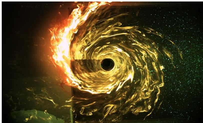
Figure 5.3: Logarithmic spiral arm of the free-surface vortex. Image captured during an initial planar laser-induced fluorescence analysis at the IT Sligo Hydraulics Research Laboratory.
