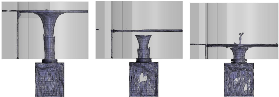
Figure 7.37: Visual presentation of the vortical structures in the flow field of a vortex chamber for the three test cases using the Q -criterion (JCR et al., 1988) (iso-surface Q = 0.05 \text{ s}^{-2} ).
